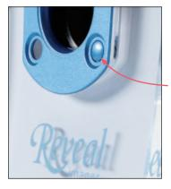
**removing the** The imaging unit (pod) should only be removed from imaging unit the upright if it is necessary to return it to Canfield for service. Otherwise, it should remain attached to the upright at all times. Before removing the unit, contact Canfield Technical Support (1-800-815-4330) for instructions on packing and returning it to our service center.
